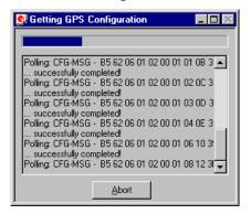
There is a window for showing the progress of data transfer to/from ANTARIS™ based GPS receivers. Clicking "GPS >> File" closes this dialog box and opens the progress window showing configurations being polled and stored into a local file. Clicking "File >> GPS" opens the same progress window showing the configurations that are sent to the ANTARIS™ based GPS receiver. This progress window closes after having finished transfer without any error.
