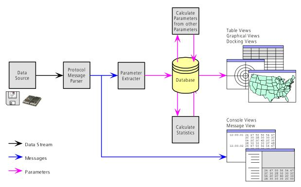
Figure 6: Engine Architecture
